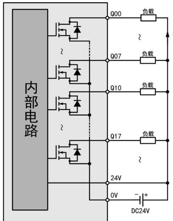
■ Source type output wiring
