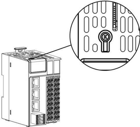
Press the multifunction button to display **E1**, keep it pressed until display **E2**, release the button within 5s, it will display **P1**, then press the multifunction button again until it appears **P2**, release the button to finish restoring the factory settings, the CPU module will restart automatically.
