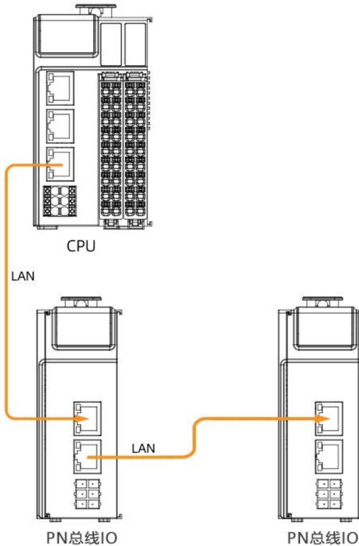
Each PROFINET device in the network is uniquely identified by its PROFINET interface. Each PROFINET interface has the following three key attributes:
