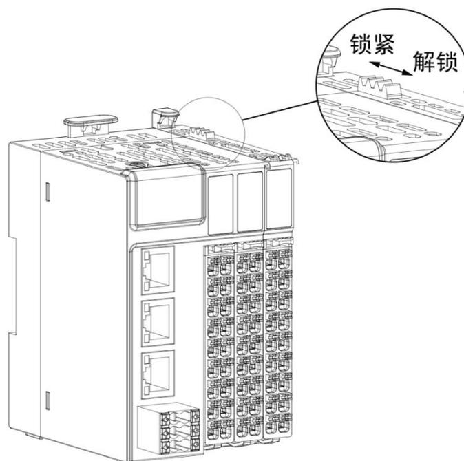
**Step 2** Pull on the module grommet bit to pull the module outward until the module separates from the base.
