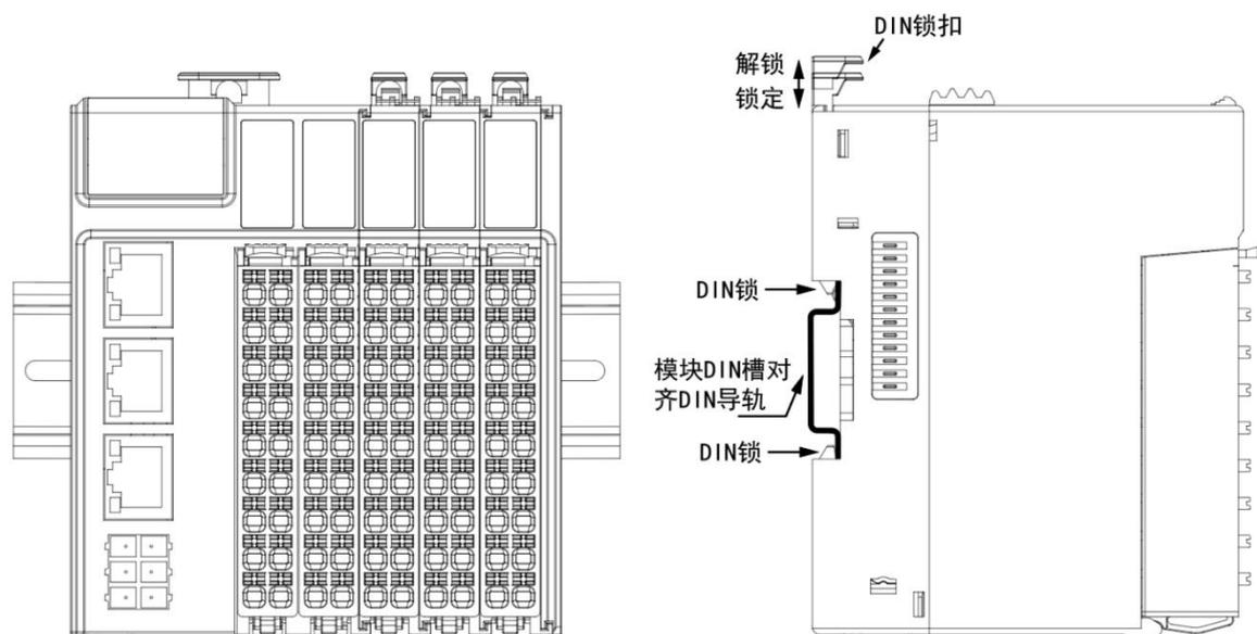
**Step 2** Install rail clamps on both ends of the rail to prevent the product from sliding on the DIN rail.
