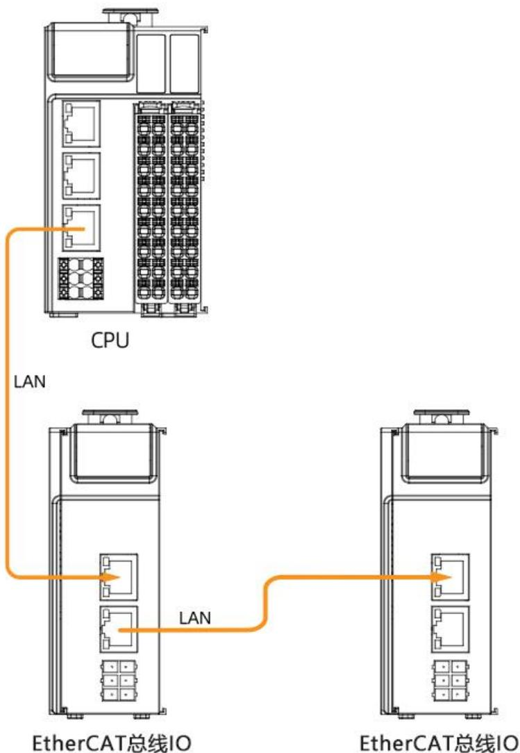
The WAC500 series can be used in combination with EtherCAT-compliant slaves to interconnect devices.
