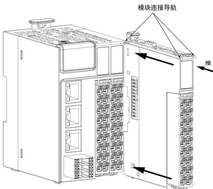
**Note :** The module and base latches should not be left unlocked for a long period of time or the latches will fail.
