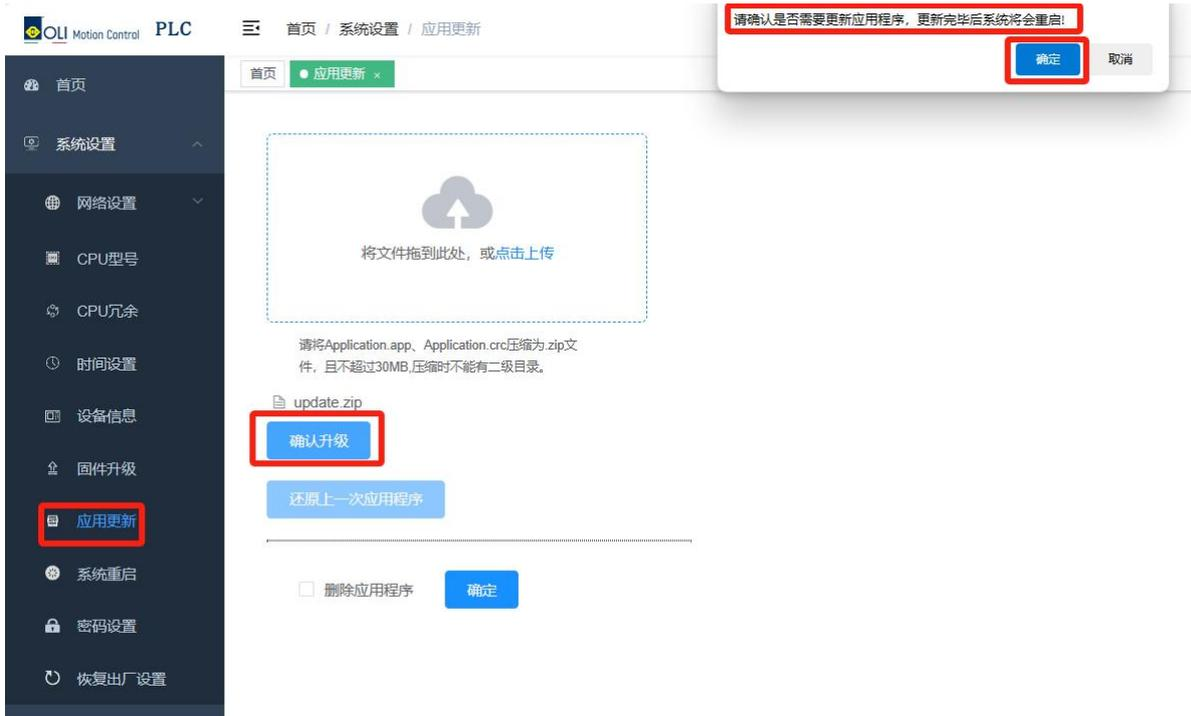
Restore last application: This operation can be performed only after the "Application update" has been performed on the web.
