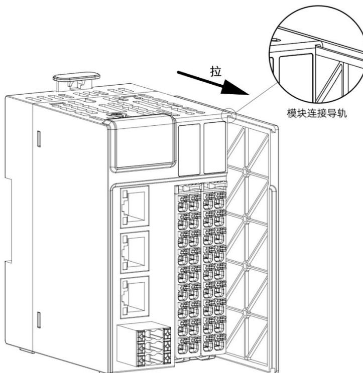
**Step 2** Align the IO module with the module connection rails of the CPU and push down on the IO module until the IO module is fully aligned with the CPU module.
