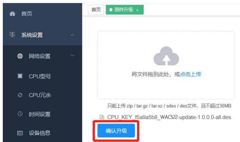
Get the upgrade key from the upgrade package to verify the upgrade operation. The upgrade key is the field after CPU\_KEY in the upgrade package name, for example, the upgrade package name is "CPU\_KEY\_f5a9a5b8\_MC522-update-1.0.0.0-all", the upgrade key is "f5a9a5b8".
