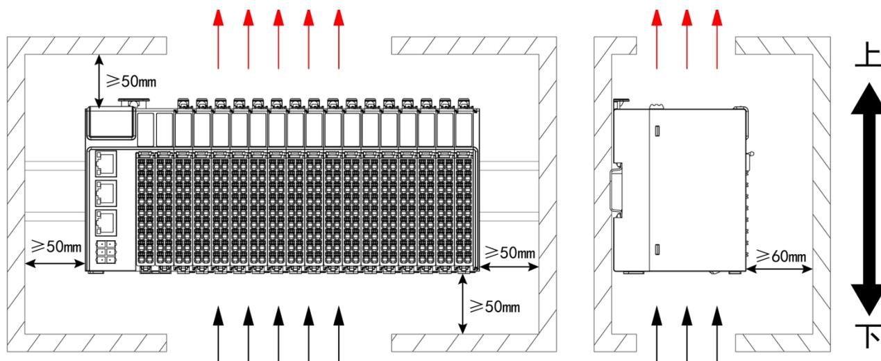
**Instruction:** If high temperature heat source equipment (heaters, transformers, large resistors, etc.) exists in the vicinity of this product, leave at least 100mm of clearance between it and the high temperature heat source equipment.
