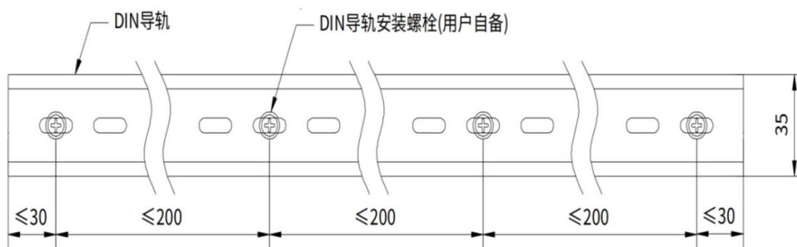
**Note :** In order to ensure the strength of the DN rail, it is necessary to install the DIN rail mounting bolts (supplied by the user) within 30mm from the end of the DIN rail, and the spacing between the 2 neighboring bolts must be within 200mm.
