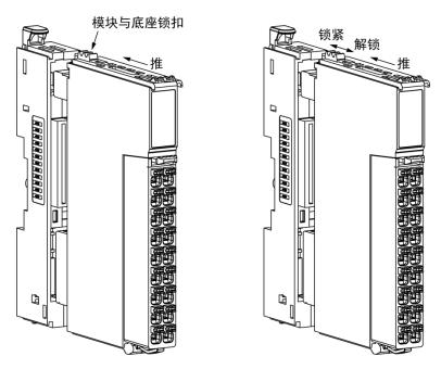
**Note**: The module and base latches should not be left unlocked for a long period of time or the latches will fail.
