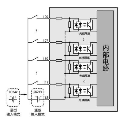
**Note**: The WL200-DI16 supports both source and drain inputs, and a single module supports only one mode.
