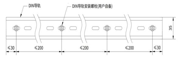
**Note**: In order to ensure the strength of the DIN rail, it is necessary to install the DIN rail mounting bolts (supplied by the user) within 30mm from the end of the DIN rail, and the interval between two adjacent bolts must be within 200mm.
