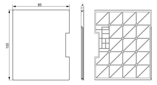
Dimensions of the product after connecting the cable (Unit: mm)
