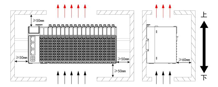
**Instruction**: If high-temperature heat source equipment (heaters, transformers, large resistors, etc.) exists around this product, keep at least 100mm of clearance between it and the high-temperature heat source equipment.
