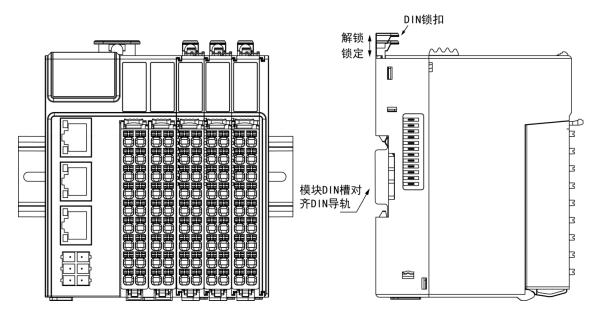
**Note**: The DIN latch must not be left unlocked for a long period of time or it will cause the latch to fail.
