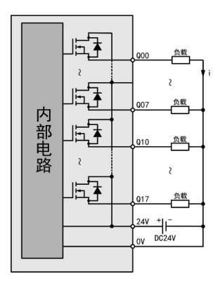
**Note**: The WL200-DQ16S output current is supplied from the external power supply terminals, and sufficient current needs to be supplied to ensure that the module output reaches the nominal output current capability.
