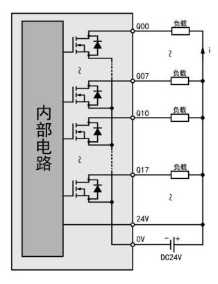
**Note**: The WL200-DQ16D requires an external 24V power supply to power the internal switching tubes, otherwise the module will not work properly.
